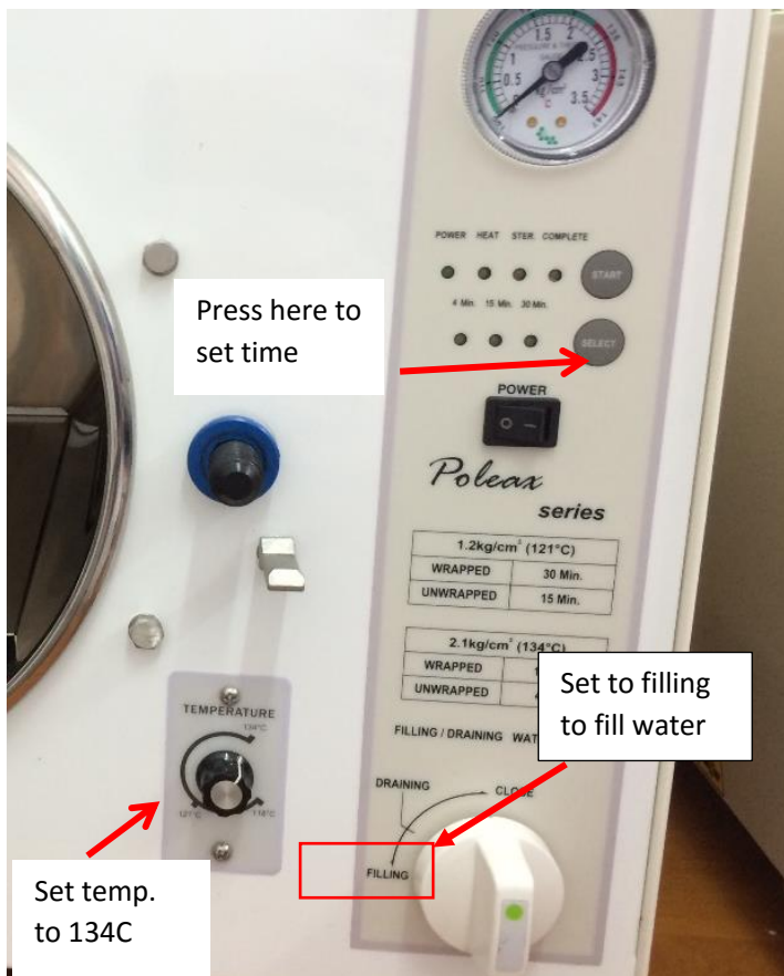
Figure 5: Autoclave SA-232X setting and preparation
