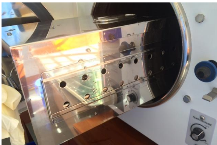
Figure 12: Insert steri box with holes open and water is filled in the chamber.
