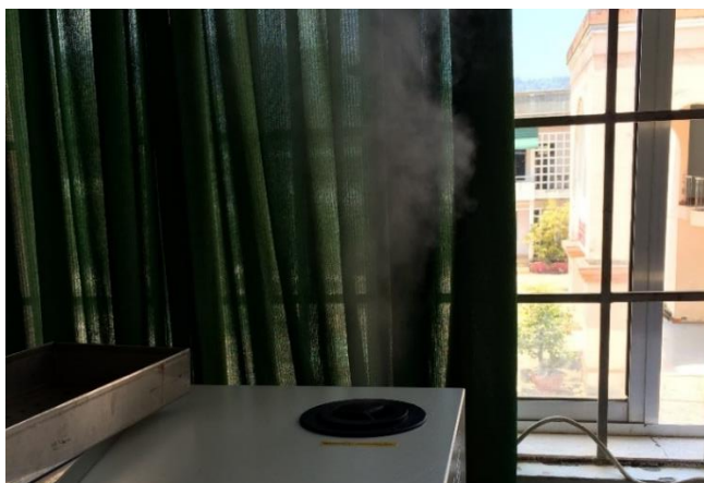
Figure 14: Steam venting from the autoclave
